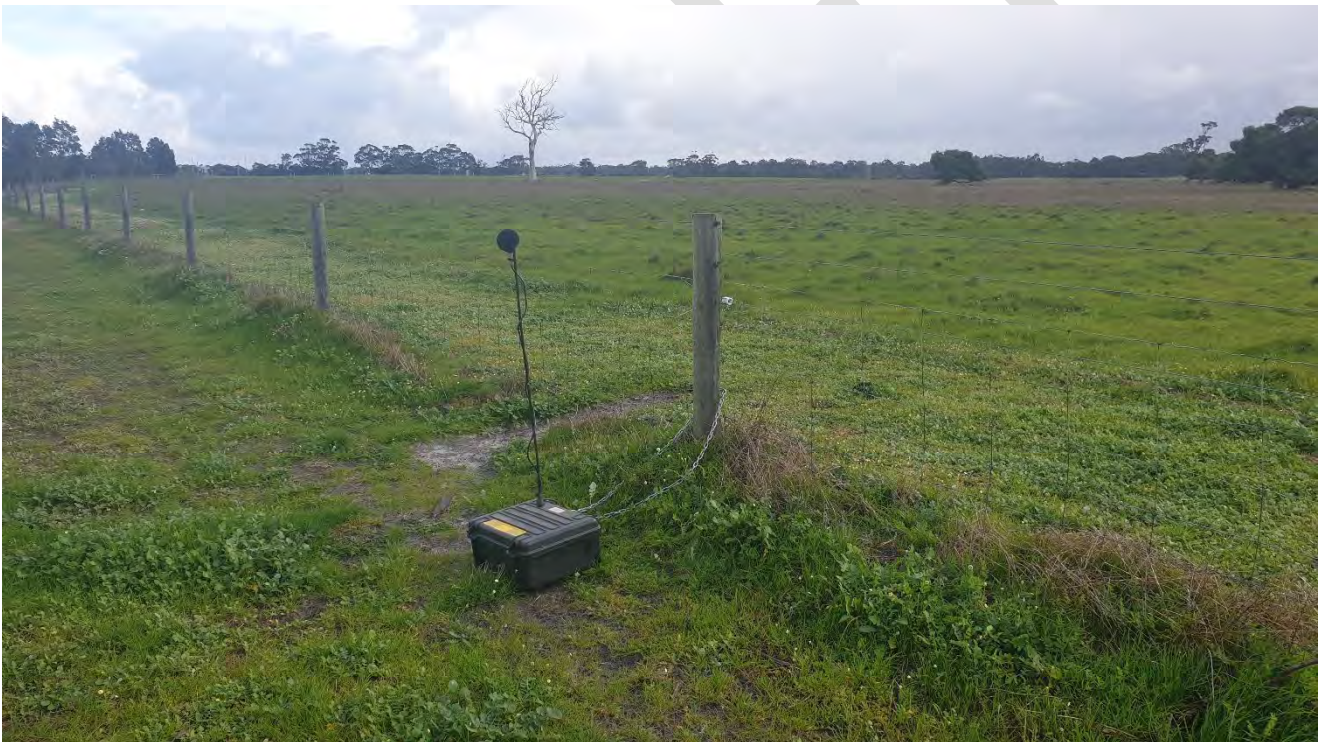
Figure 3-1: Photograph of Sound Level Meter on Site
